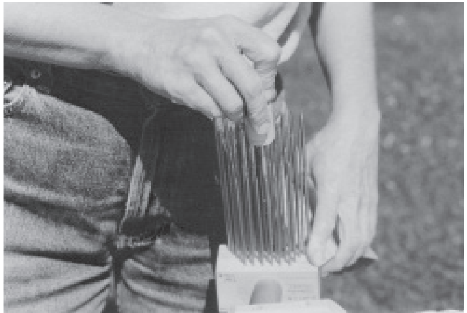
These steel combs are used to straighten wool fibers in preparation for spinning. Running the wool through the combs also removes any debris left after washing. Photo: Jill Breit
